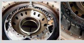
**SUPERIOR CLEANLINESS:** The bearing housing on the left is from a CFM56 engine that used ASTO 560. It is visibly cleaner than the housing on the right, which operated with a competitor's oil for a similar number of hours.
